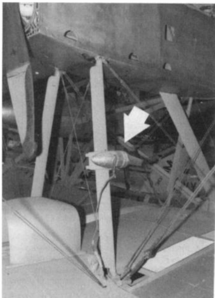
Figure 5. The propeller-driven generator (see arrow) for the transmitter is mounted to the center engine strut.
